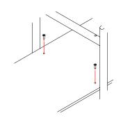
5. When the shelf is in place, fix the screws in all six holes, loosely.
